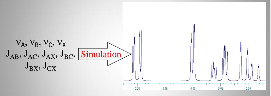
There is no explicit way to transform spectrum I(v) to spectral parameters – but that can be done iteratively: guessing trial parameters, simulating spectrum with them and then trying to improve (iterate) the guess.
