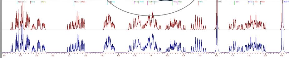
28 protons, 24-spin particles, 8 sub-systems => 688 transitions, only ! Simulation time ca. 2 s.
