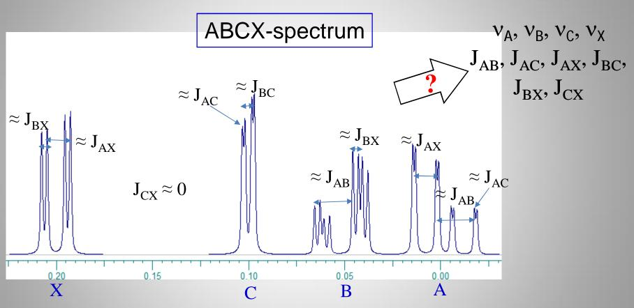
Chemical shift = weight point of multiplet Coupling constant ≈ difference of two lines
